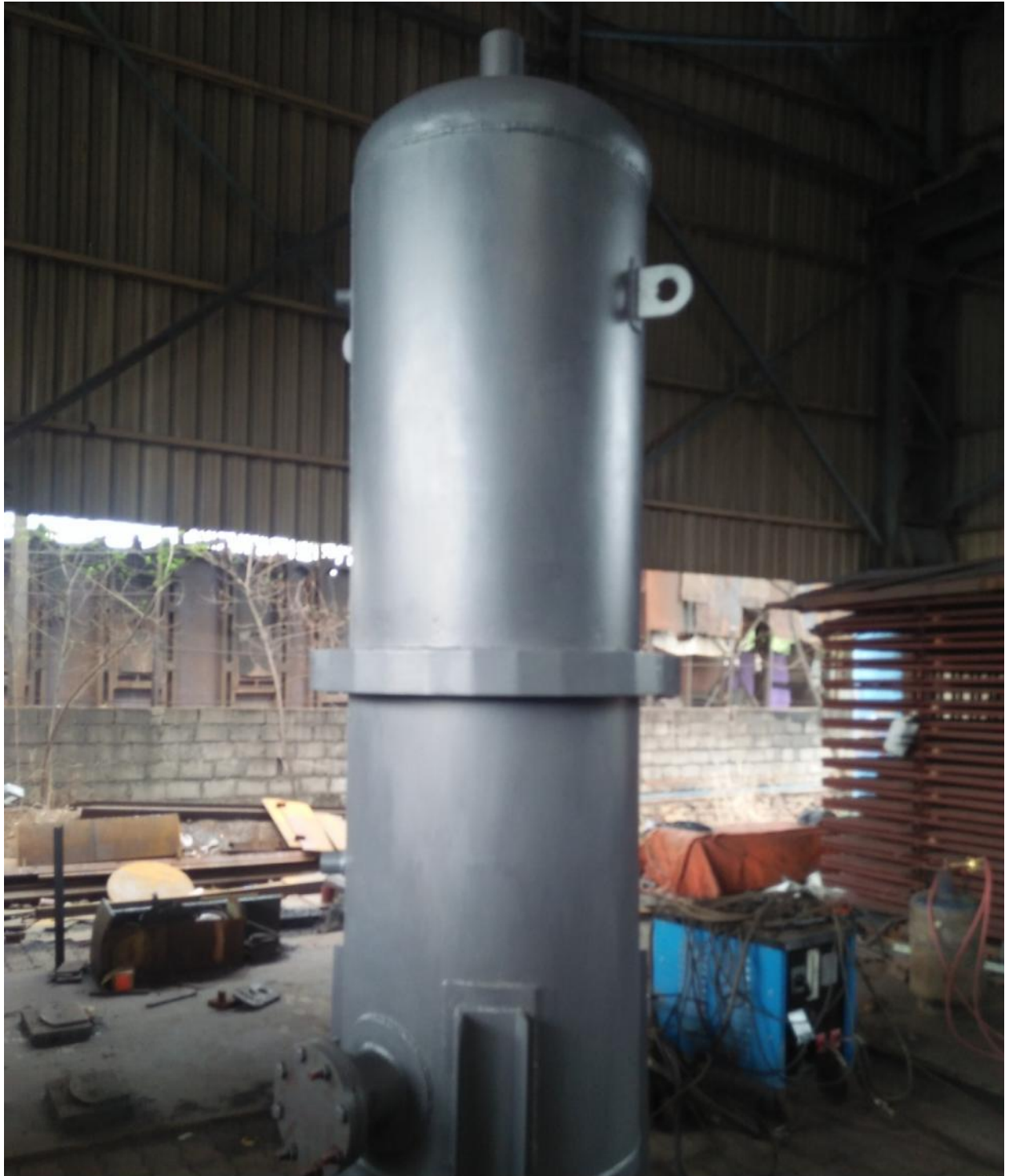
CONTINEOUS BLOW DOWN TANK
